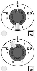
The grill has two elements that allow either the whole area of the pan to be heated or just the right hand half.
